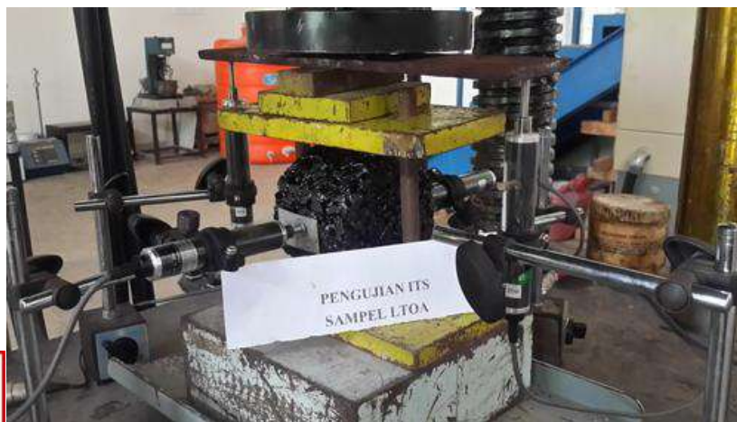
Gambar 7. Pengujian indirect tensile strength
