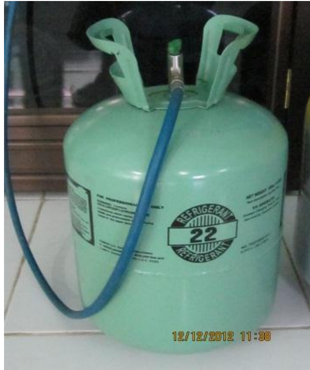
Gambar A.1 Refrigeran R22
