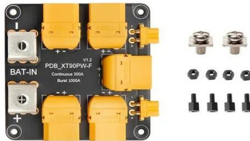
Figure 40. Power Distribution Board (PDB)
