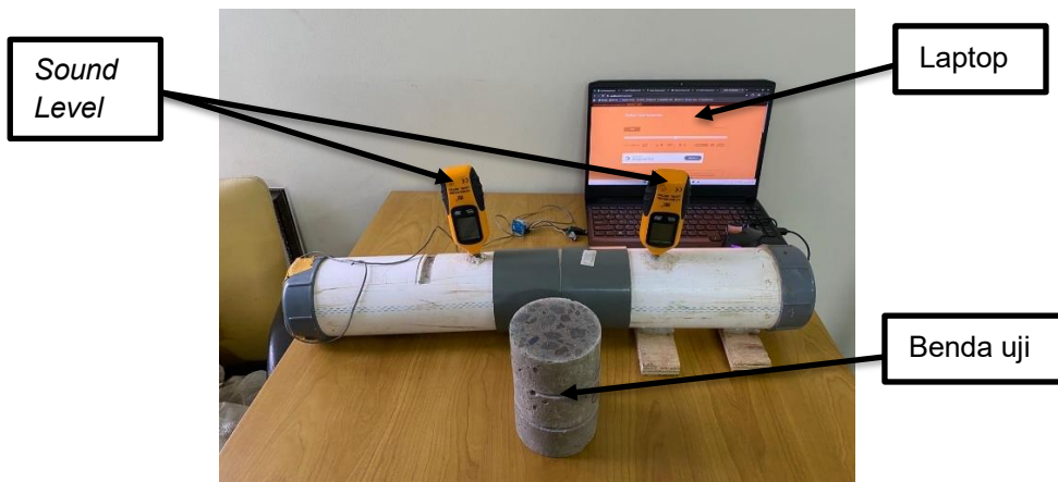
Gambar 6. Pengujian Sound Absorption Coefficient (SAC) Beton
