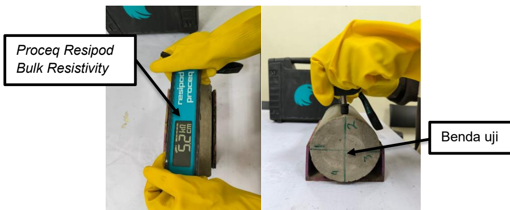
Gambar 7. Pengujian Resistivity Beton
