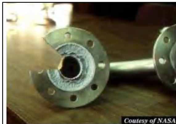
Gambar 10. Crevice corrosion ( Budi Utomo,2009 )
