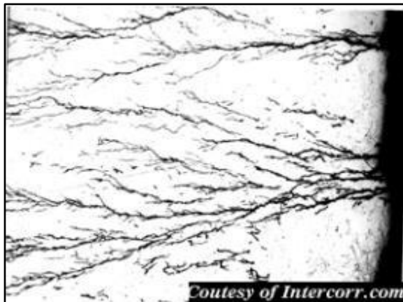
Gambar 9. Stress corrosion ( Budi Utomo,2009 )
