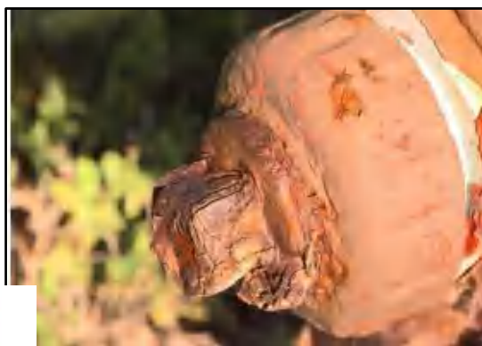
Gambar 12. Fatigue Corrosion ( Budi Utomo,2009 )
