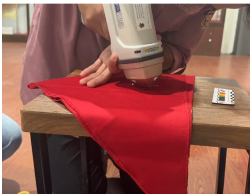
Gambar 11. Analisis XRF Portable di Museum Karaeng Pattingalloang (Dok. Wandu, 2025)
