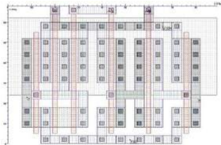
Gambar 11. Half Adder Layout 2.
