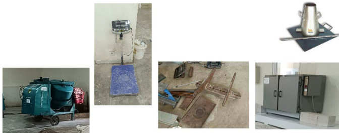
Gambar .12. Alat-alat ; concrete mixer, timbangan, tumpuan baja, kerucut abrams, oven
