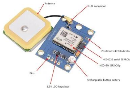
Gambar 8 Pinout Modul GPS Neo-6m (sumber: Arta et al., 2022)
