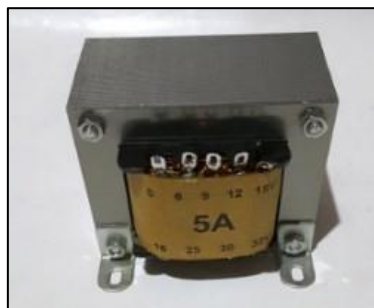
Gambar 14 Trafo Non-CT 5A
