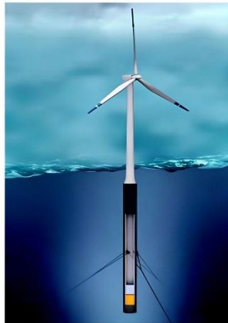
Gambar 3. Sistem tambat taut ( http://www.builtworlds.com/news/2016/1/22/worlds-first-floating-wind-farm-to-surface-off-scottish-coast ) diakses pada tanggal 29 Oktober 2024
