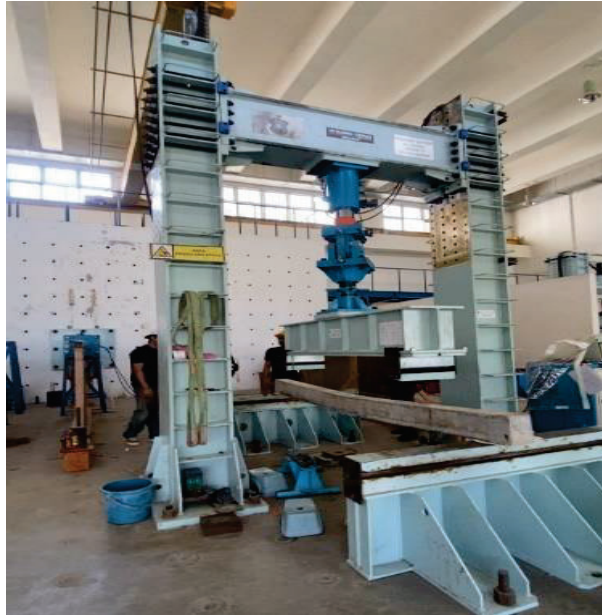
Gambar 2.19. Static loading frames
