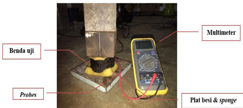
Gambar 8. Pengujian Electrical Resistivity
