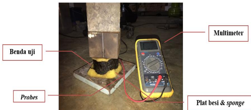
Gambar 8. Pengujian Electrical Resistivity
