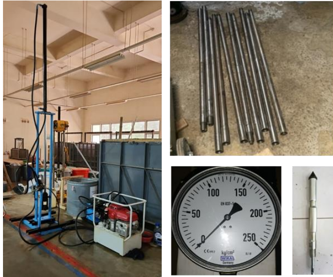
Gambar 9. Alat uji CPT ( Cone Penetration Test )
