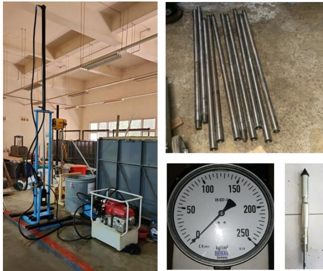
Gambar 10. Alat uji CPT ( Cone Penetration Test )
