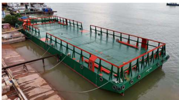
Gambar 7. Deck Cargo Barge 250x80x14 ft
