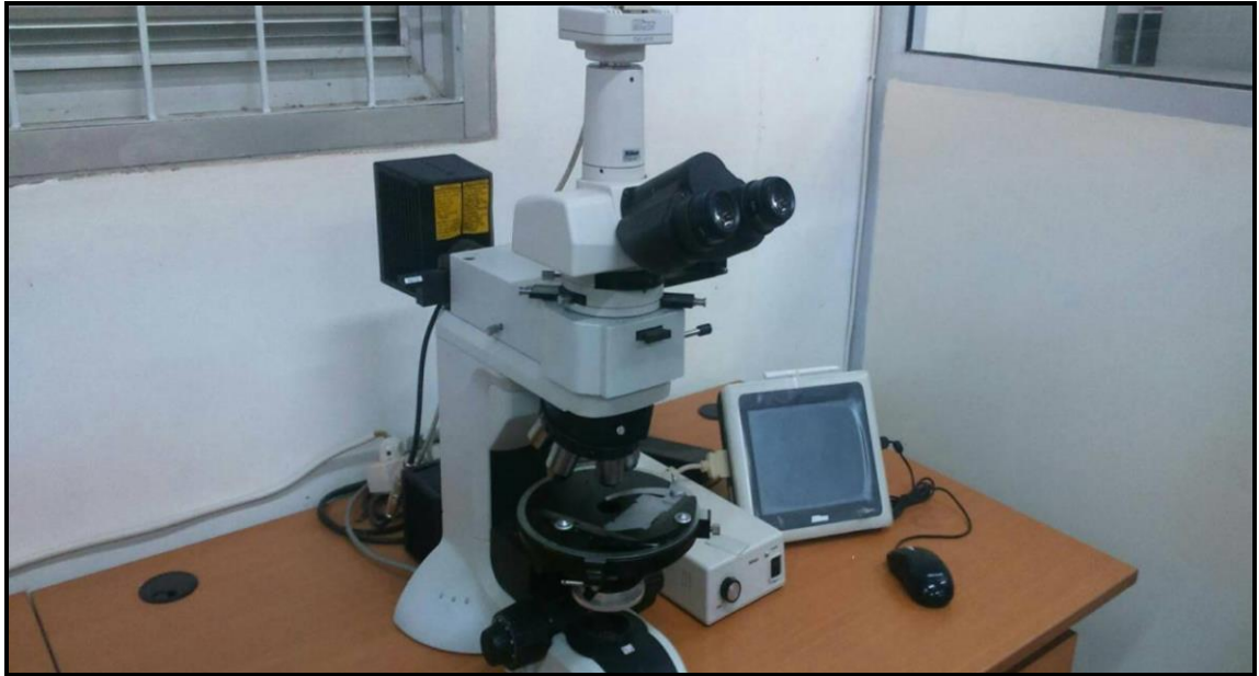
Gambar 3.5 Mikroskopis tipe Nikon Eclipse LV 100N POL
