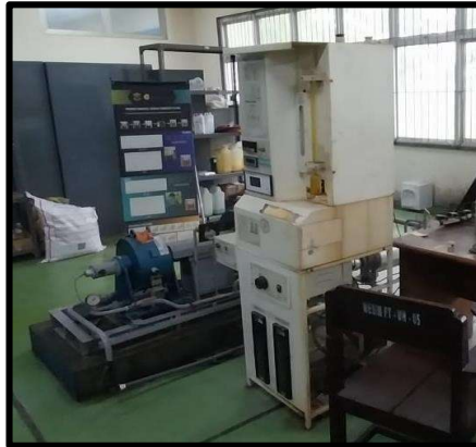
Gambar 8. VCR Engine Test Setup
