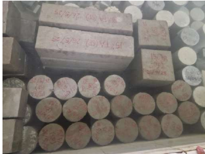
Gambar 10. Curing Air Benda Uji
