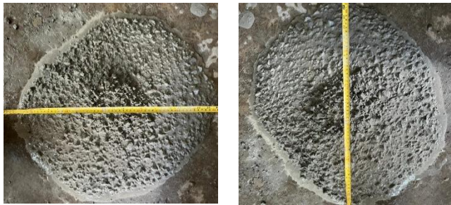
Gambar 5. Pengujian slump flow
