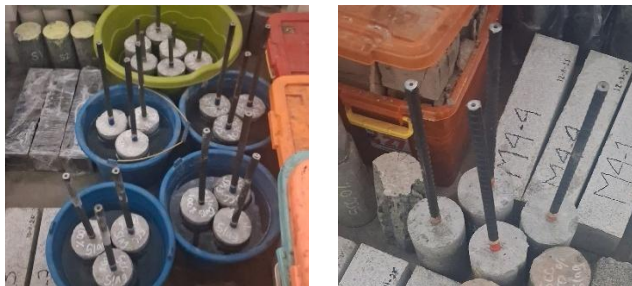
Gambar 6. Proses curing benda uji
