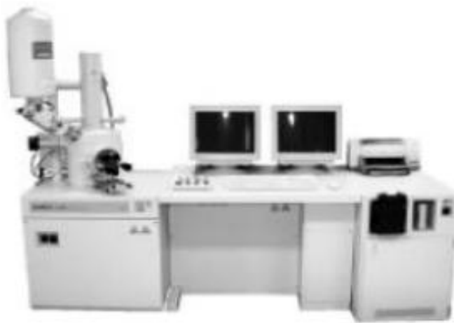
Gambar 5. The SEMEDX Integrated System (Martinez, 2010)
