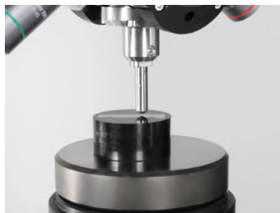
Gambar 2.14 Pengujian Vickers hardness (Sumber: https://emcotest.com )
