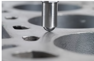
Gambar 2.12 Pengujian Brinell hardness (Sumber: https://emcotest.com )
