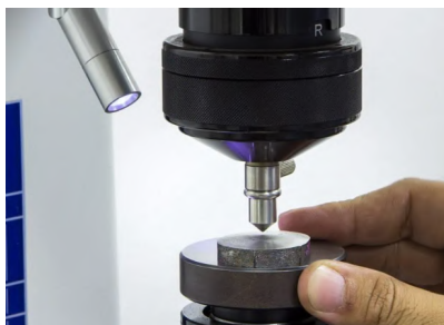
Gambar 2.16 Pengujian Rockell hardness (Sumber: https://xometry.pro )
