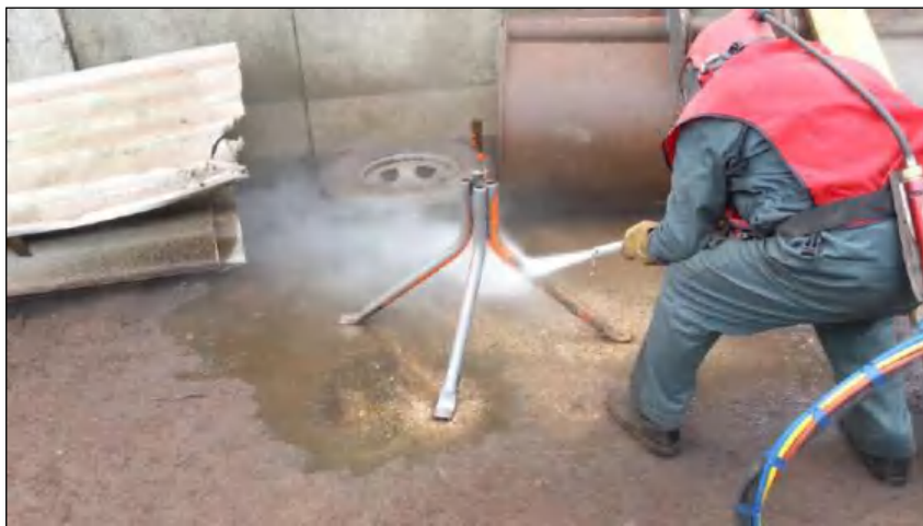
Gambar 3. Wet Sandblasting Process (Sumber: storage.googleapis.com )
