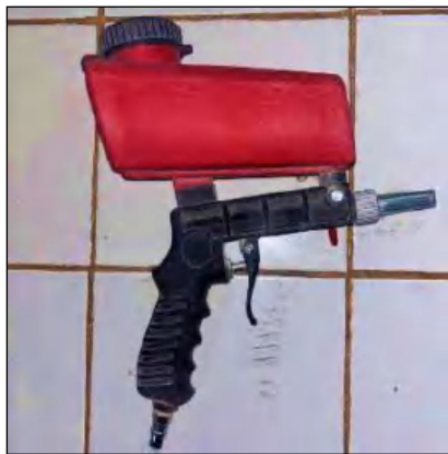
Gambar 6. Nozzle Blasting/Blasting Gun
