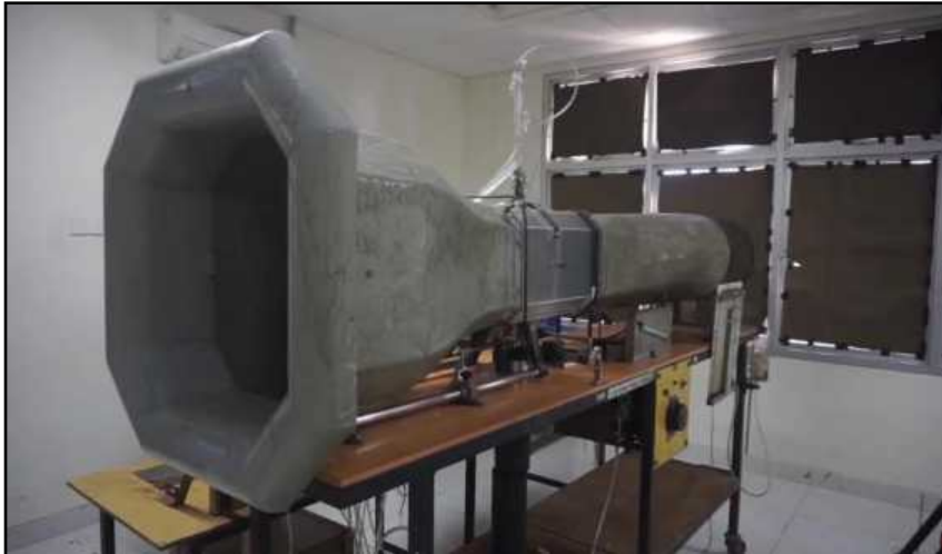
Gambar 18 Terowongan angin (Wind tunnel).
