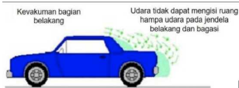
Gambar 6 Rear Vacuum Daerah Belakang Mobil (Azizi, 2010)
