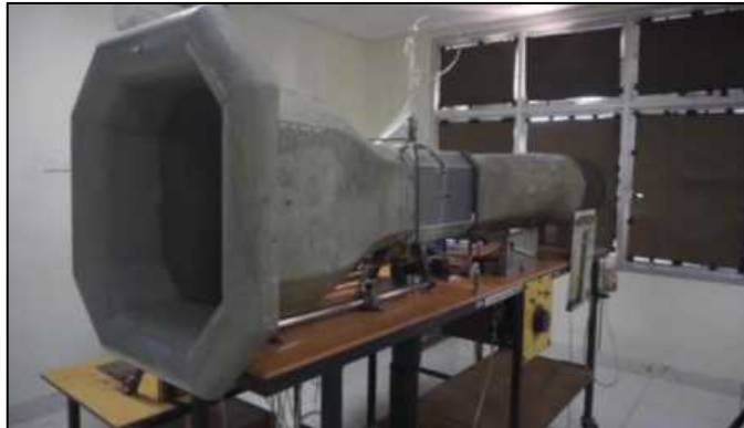
Gambar 15 Terowongan Angin ( Wind Tunnel )
