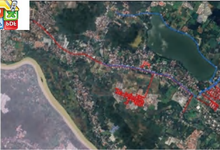
Gambar 14. Layout Jaringan Pipa Distribusi PDAM Bontomarannu Section 1
