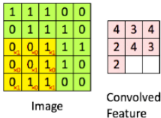
Gambar 3 Proses convolution (Khan et al. , 2018)
