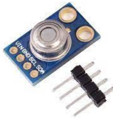
Gambar 10. Sensor Suhu MLX90614
