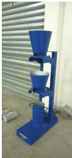
Gambar 3 Compacting factor concrete
