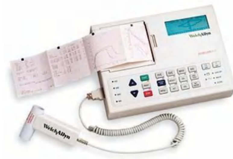
Gambar 2. Alat spirometer berbasis komputasi (autospirometer)
