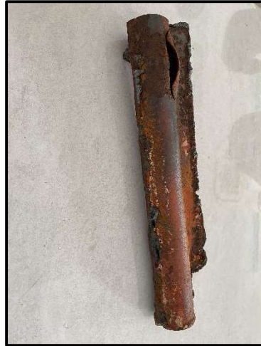
Gambar 1. Spesimen Wingwall Superheater Tube 20G
