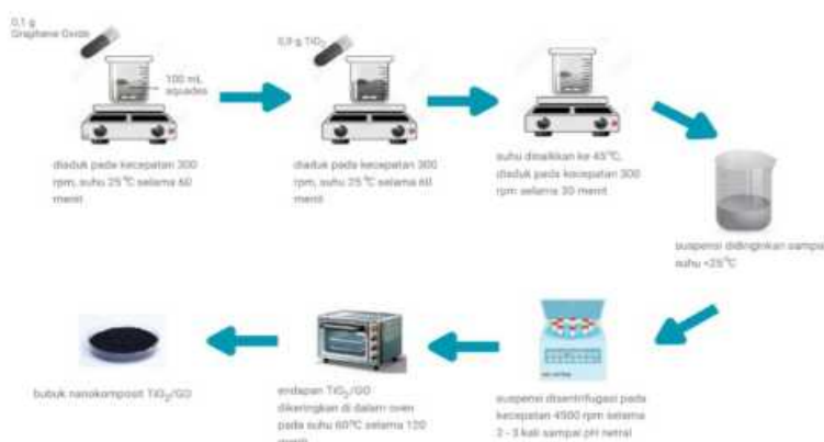
Gambar II.2 Sintesis nanokomposit \text{TiO}_2/\text{Graphene Oxide} dengan metode Mechanical Mixing
