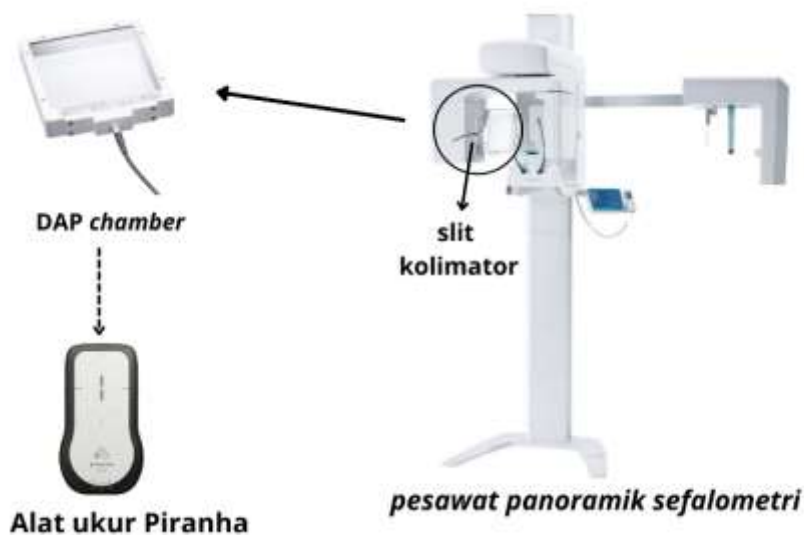
Gambar 7. Tahapan Uji Dose Area Product (DAP) (RTI, 2025; Trident, 2024)
