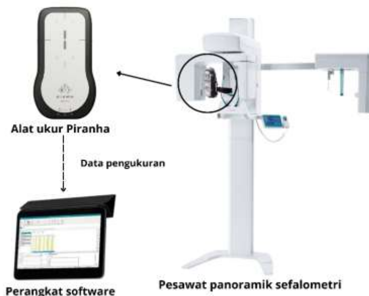
Gambar 5. Tahapan uji generator tabung (RTI, 2025; Trident, 2024)
