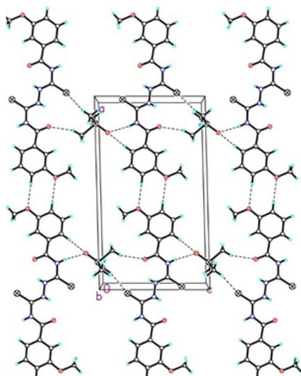
**Figure 7:** Molecular packing of compound 2 viewed down b axis. The hydrogen bonds are illustrated by the dashes lines
