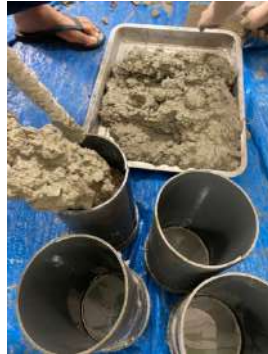
Pengecoran Beton Segar Kedalam Bekisting Pipa
