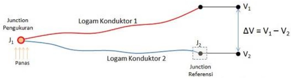
Gambar 2.7 Typical Rangkaian Thermocouple
