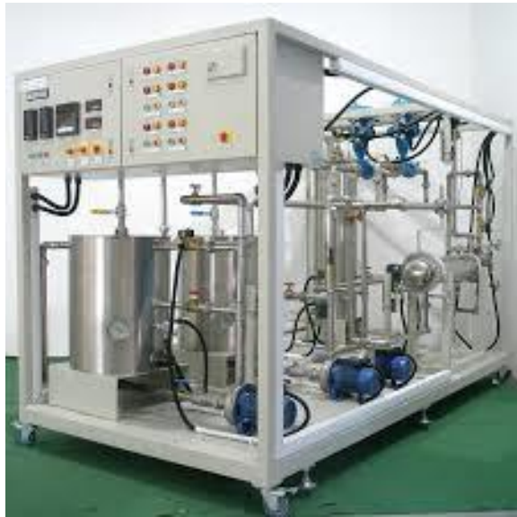
Gambar 2.1 Alat Boiler heating batching control trainer ( Model : Se 107)
