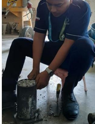
A photograph of a person wearing a blue t-shirt and dark pants, kneeling on the floor. They are working on a single cylindrical metal mold, which appears to be partially filled with a material. The person is using their hands and a tool to manipulate the contents of the mold, likely preparing to remove it from the mold or adjust its position.               | Membuka cetakan benda uji    |
