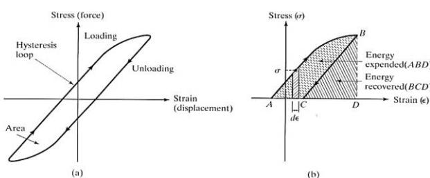
**Gambar 2.8 : Diagram Stress-Strain (Dewanto et al., 1999)**
