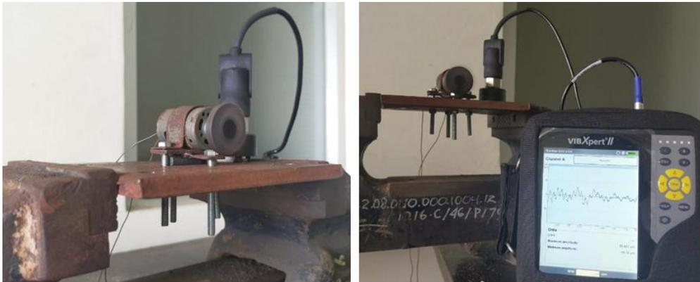
**Figure 3.** Set up installation for vibration test
