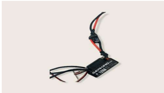
Gambar 3.14 ESC( Elektronic speed control )
