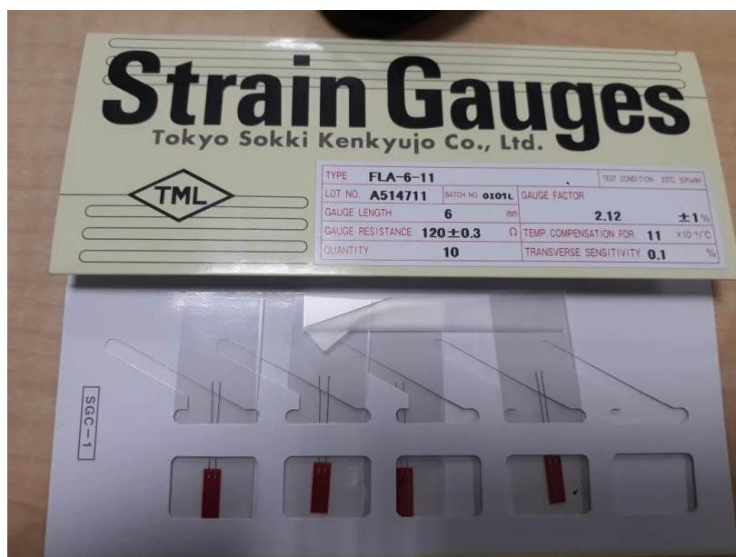
Gambar 11. Jenis Strain Gauges
