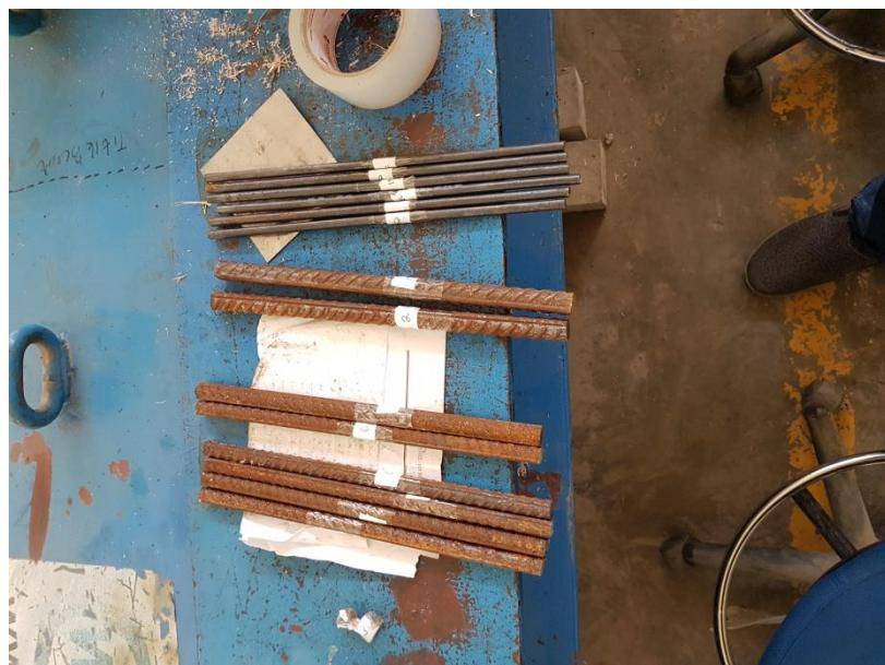
Gambar 5. Benda uji test tarik besi tulangan ( $\varnothing 8$ , D13, D16)
