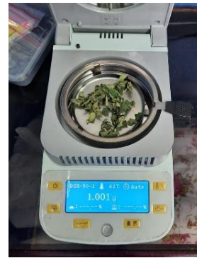
Pengujian kadar air metode moisture analyzer
