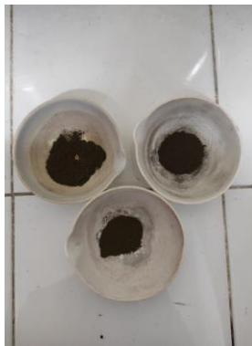
Pengujian kadar air metode oven
