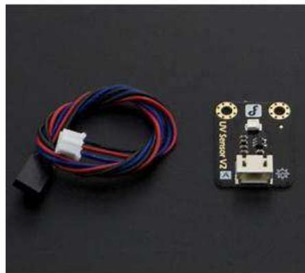
Gambar 2.7 Sensor UV V2
