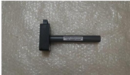
**Gambar 2.5** Konduktivimeter (sumber [http// eprints. uny. ac.id/30252/bab%202.pdf](http://eprints.uny.ac.id/30252/bab%202.pdf))
