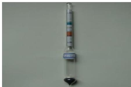
**Gambar 2.4** Salinometer (<https://www.scribd.com/document/356419891/datasheet-sensor-konduktivitas-kadar-garam-tds>)
