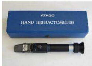
**Gambar 2.3** Refraktometer (<https://www.scribd.com/document/356419891/datasheet-sensor-konduktivitas-kadar-garam-tds>).
