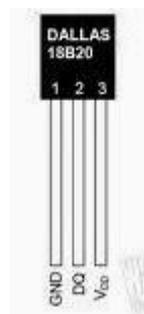
**Gambar 2.9** Pin Sensor Temperatur ( <http://www.sunrom.com>)
