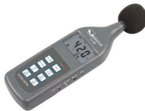
Gambar 2.1 Sound Level Meter
