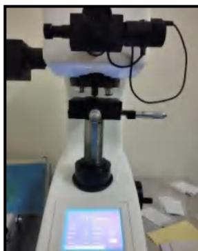
**Gambar 28.** Vickers Hardness Tester
