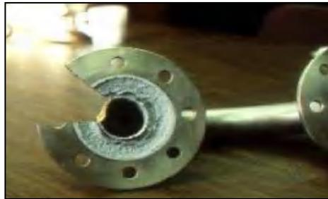
**Gambar 8.** *Crevice corrosion*
