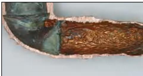
**Gambar 5. Erosion corrosion**
