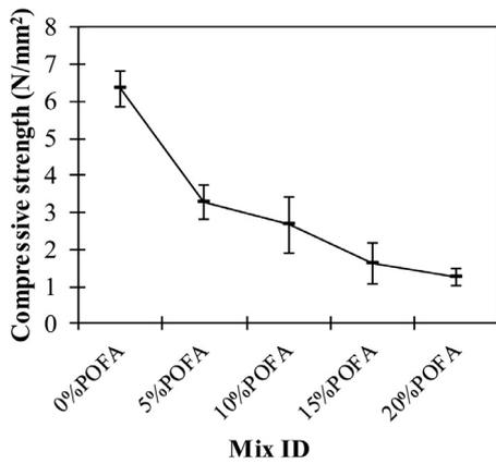
Fig. 9. Compressive strength of bricks.
