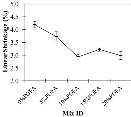
Fig. 5. Brick linear shrinkage.
