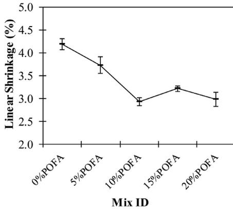
Fig. 5. Brick linear shrinkage.
