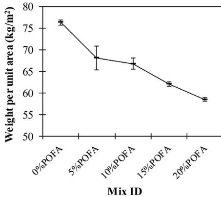
Fig. 6. Weight per unit area of brick specimens.
