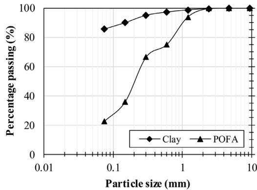
**Fig. 3.** Particle size distribution of clay and POFA.
