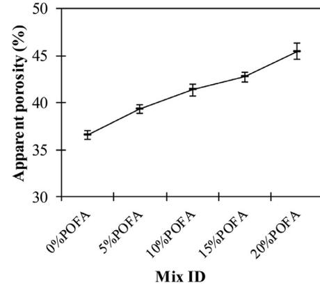
Fig. 7. Apparent porosity of brick specimens.
