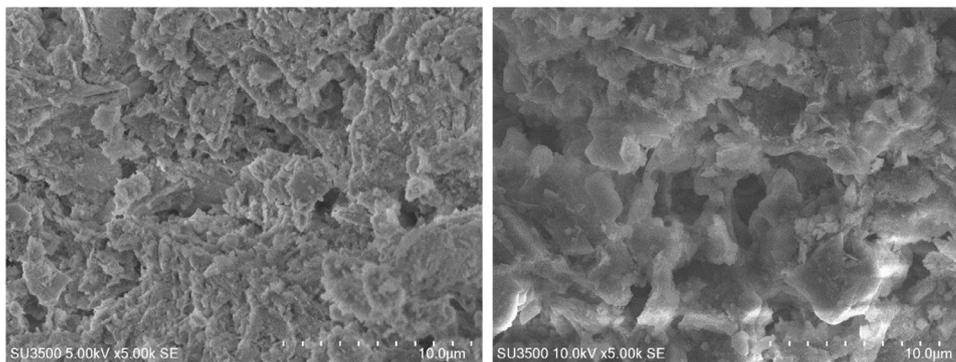
Fig. 12. SEM images of bricks with POFA contents of (a) 0% and (b) 10%.
