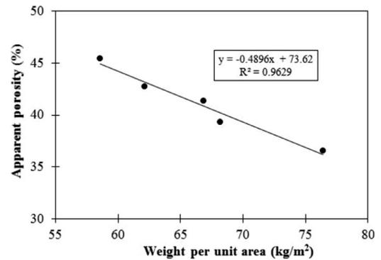
Fig. 8. Relationship between the apparent porosity and the weight per unit area of brick specimens.
