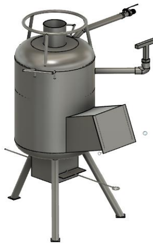
Gambar 2. 16 Tungku Biomassa Injeksi Uap
