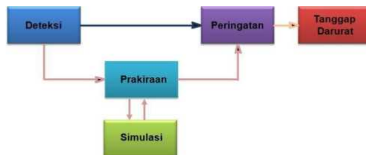
Gambar 1 Konsep Flood Early Warning System (FEWS)
