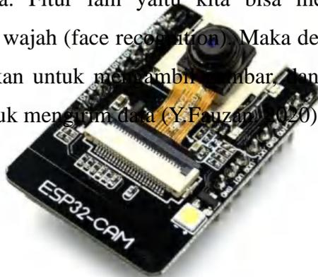
Gambar 2 ESP32-CAM
